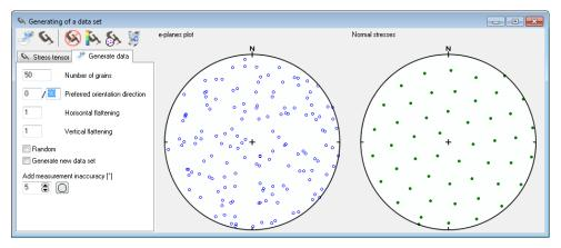
button generates a data file according to settings on Generate data tab (figure  $\uparrow$ ). The user can set the number of grains, direction and degree of preferred orientation of grains and finally the method of *c*-axes generation – with perfectly uniform or random distribution ( $\square$  Random). Measurement error can be introduced into the data file by pressing  $\boxdot$ . *c*-axes can be input also directly by left-clicking into the *c*-axes plot (*e*-planes are generated randomly).
